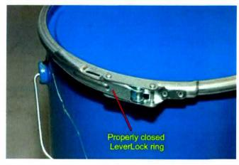
**Step 8**--Insert the tamper-evident T-clip through the slot in the lever. This will hold the lever in place. The T-clip should also pass through the loop attached to the body of the ring.
