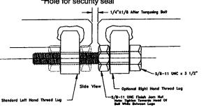
To ensure proper closure, do not exceed ring closure gap.
